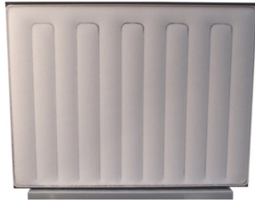
Laser-welded Flat Plate Membrane during Pressure Test
